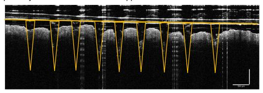
Figure 3 - B-Scan OCT image of microneedle array in skin - microneedle shape highlighted by yellow
