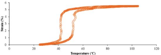
Fig. 1: Early hysteresis loop of a NiTi alloy subjected to thermal cycles and 150 MPa stress. Temperature is measured with IR temperature sensor.
