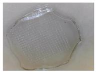
Figure 2 - Microneedle array structure consisting of 324 needles of height 750  $\mu$ m, base diameter 200  $\mu$ m, tip diameter 10  $\mu$ m and centre-to-centre spacing of 600  $\mu$ m
