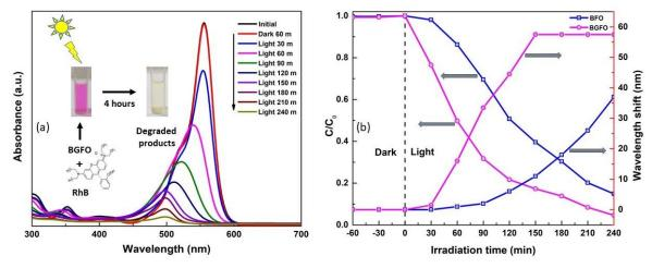
Fig: (a) Spectral changes during the degradation of RhB dye in the presence of BGFO nanoparticles under solar irradiation and (b) A plot of degradation (%) vs irradiation time (min) for BFO and BGFO nanoparticles (black Y axis) and corresponding wavelength shifts in the absorbance band of RhB (red Y axis).
